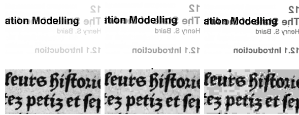
Figure 1. First row : Different levels of bleed through intensity (from left to right : low, medium, high). Second row : different levels of JPEG compressions
